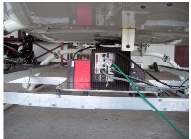
Fig.: RGB-camera, Airborne Laser Scanner (ALS), of Inertial Navigation System (INS)
